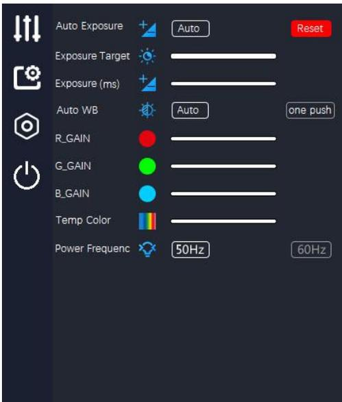
Move the corresponding bar to adjust the parameters. The user can adjust the image brightness with manual operation to adjust target brightness and exposure time if auto exposure and auto white balance is not correct.
