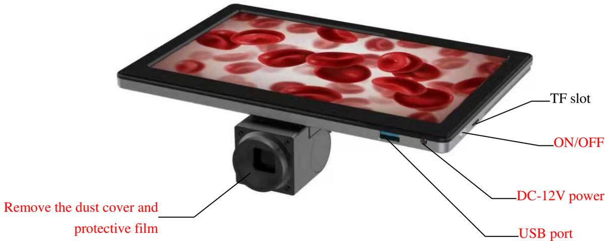
2.1.1 Remove the dust cover and the plastic cover film in the screen and put the screen to the C-mount.
